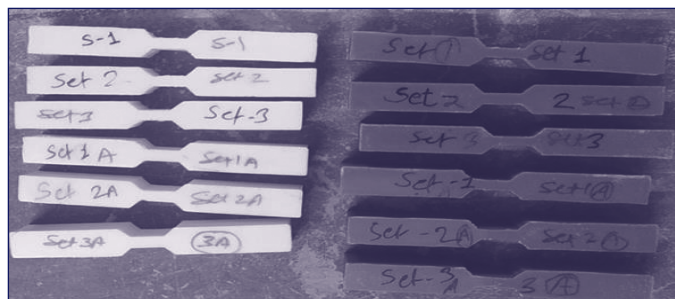
Figure 5. Tensile test specimen and sizes. [15]
